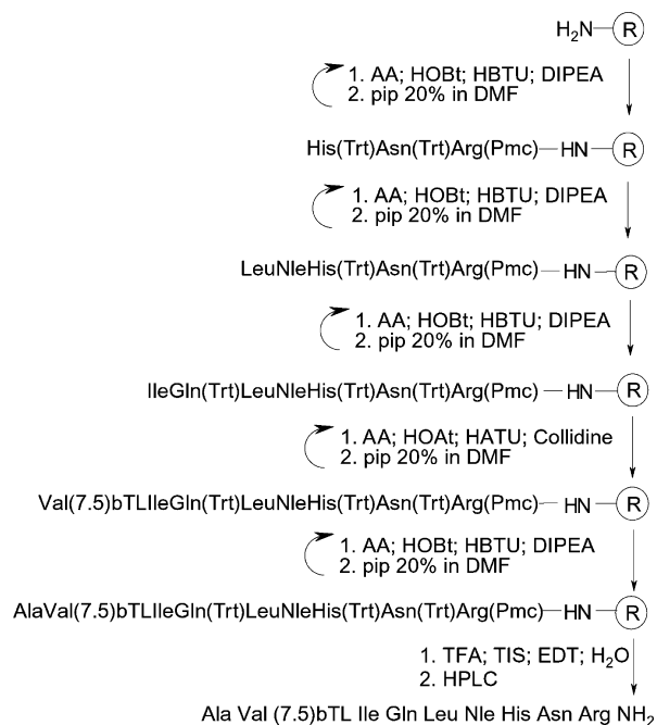
Scheme 1 Solid-phase synthesis of analogues I-III (analogue I is reported as an example of the synthetic protocol).
